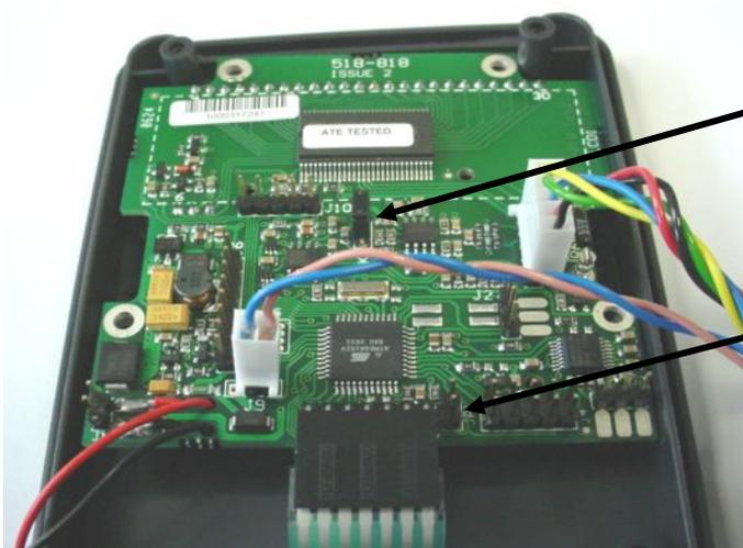
Sensitivity link should be in this position for use with sensors, with sensitivities  $\leq \pm 5\text{mV/V}$
