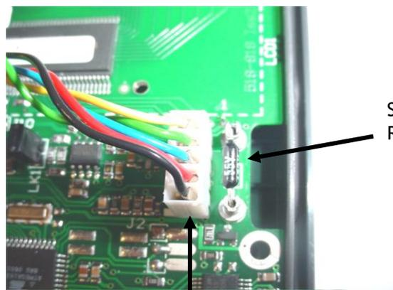
Shunt Calibration Resistor
