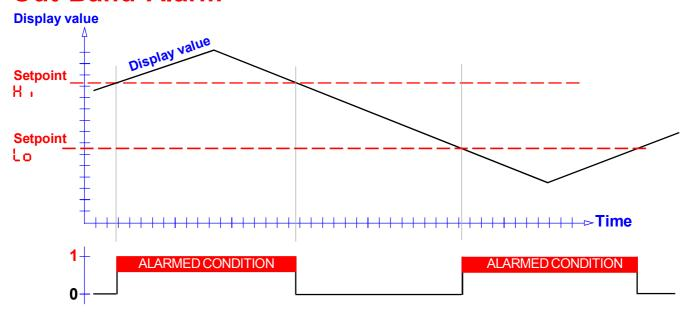
The Setpoints can be placed anywhere you like, in the range 89999 to +999999 and will include a decimal point in the appropriate position if you have set your display range to have a decimal point.
